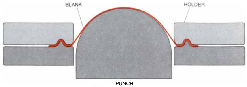
**STRETCHING** is the second major mode of forming sheet metal by stamping. It is illustrated here by a punch-stretch test that is employed in the laboratory to assess the deformation of a piece of sheet metal during stretching. A metal blank (color) is clamped firmly at the edges and then stretched over a hemispherical punch. The groove in the upper die and the bead in the lower one ensure that there is no drawing in of metal, so that the test assesses only stretching.
