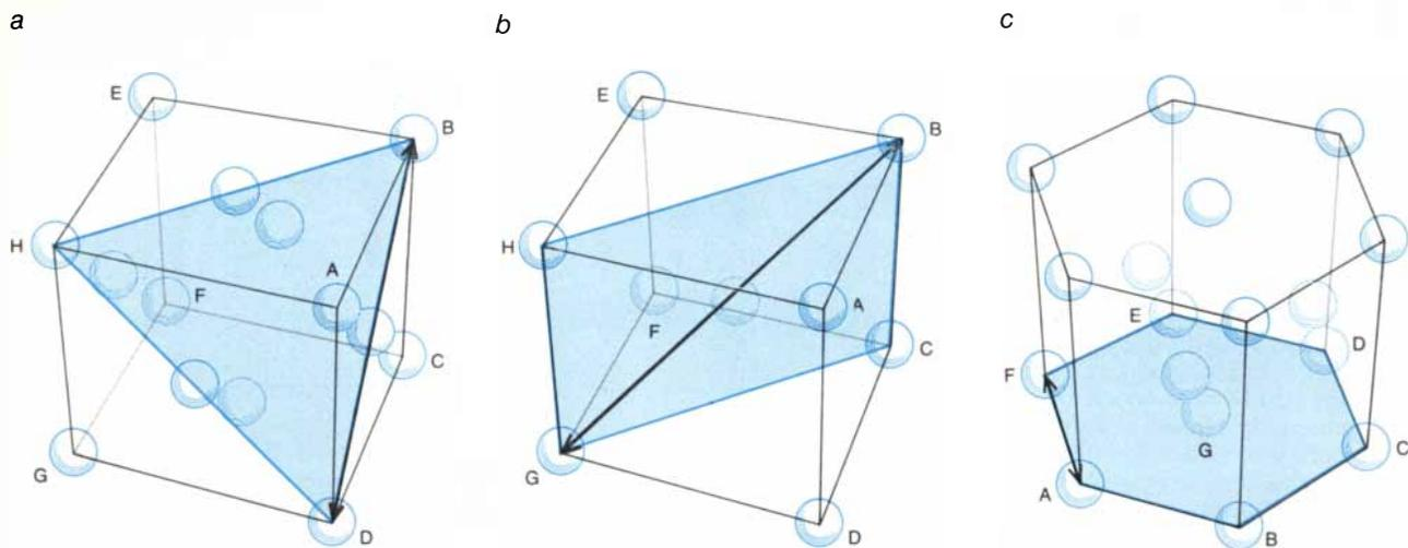
**CRYSTAL STRUCTURES** commonly found in metals are depicted. They are face-centered cubic (a), with an atom at each corner of the cube and one at the center of each face; body-centered cubic (b), with an atom at each corner and one in the center of the cube, and hexagonal close-packed (c). The structure affects the ability of a
