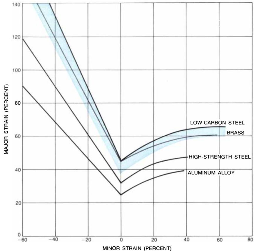
**FORMING-LIMIT DIAGRAM**, obtained by deforming metals in tests, indicates whether a metal can be shaped without risk of failure, or tearing. The broad colored band represents steel; under strains in the region below the band steel can be expected to undergo forming successfully, whereas above the band the strains probably will cause the metal to fail during forming. The curves for other metals are less firmly established by experience than the steel curve is.
